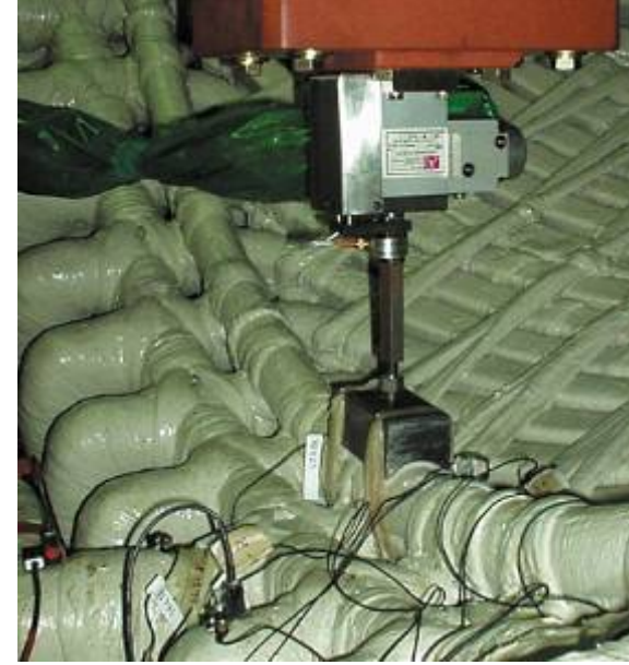
Stator End Winding Vibration Test Equipment
