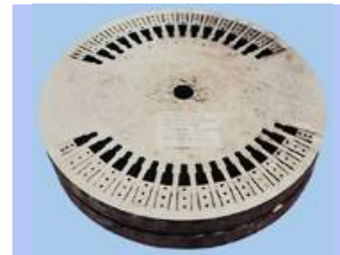
Spinning Burst Test Using Full -Size Rotor
