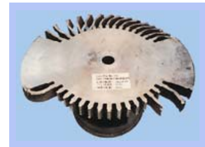
Spinning Burst Test Using Full -Size Rotor
